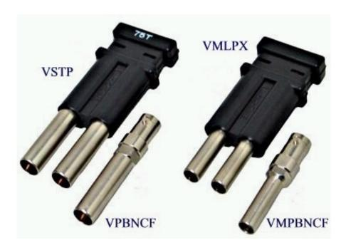
Switchcraft increases its line of video patching products with three new adaptor accessories. The dual looping plug series allows single or dual isolated video jacks to normal a signal path through. Designed for 75 Ohm applications, the looping plugs are available in Standard (WECo .090 pin) or Midsize (Mini-WECo .048 pin).
