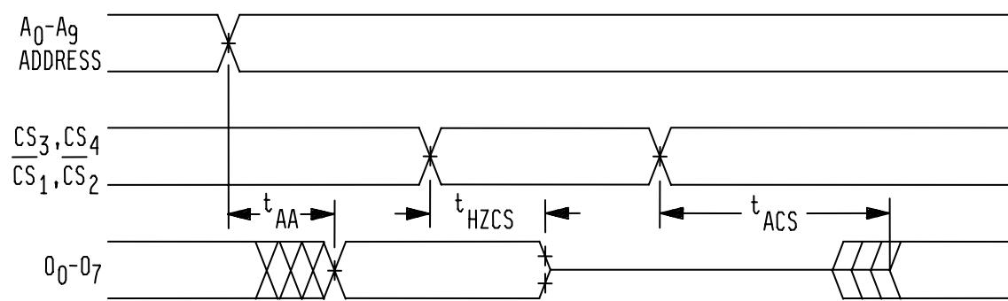
FIGURE 4. Switching waveforms.
