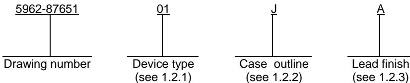
1.2.1 Device type(s). The device type(s) identify the circuit function as follows:
