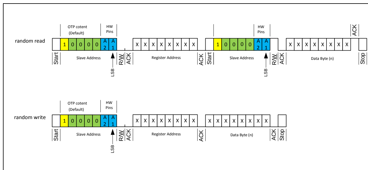
Figure 32: Slave Address Construction
