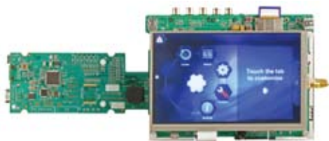
QNX® Software Systems Neutrino® RTOS and Aviage® Middleware Suite on the MCIMX35LPDK
