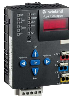
Modular buscoupler CANopen CE; Approvals: US in preparation
