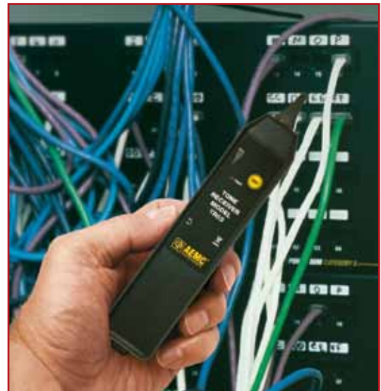
Model TR03 used to find cables in a panel.
