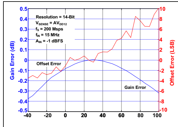
FIGURE 3-22: Gain and Offset Error Drifts vs. Temperature using Internal Reference, with Respect to 25^\circ\text{C} : f_S = 200\text{ Msp} s.
