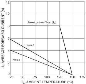
Fig. 6 Forward Current Derating Curve
