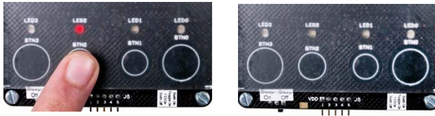
Figure 3-11. Kit with Delay Off Feature Disabled
