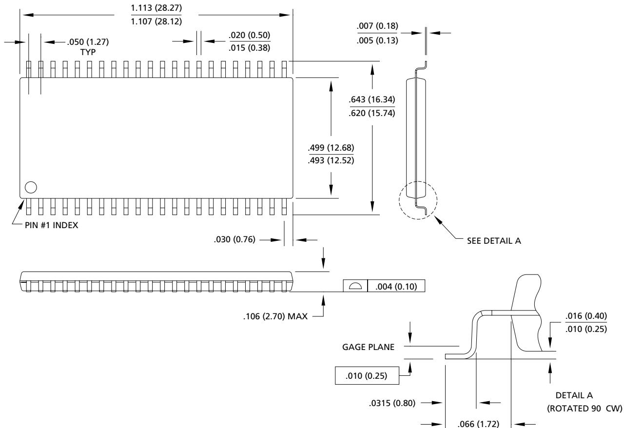
**NOTE:** 1. All dimensions in inches (millimeters) MAX or typical where noted.
