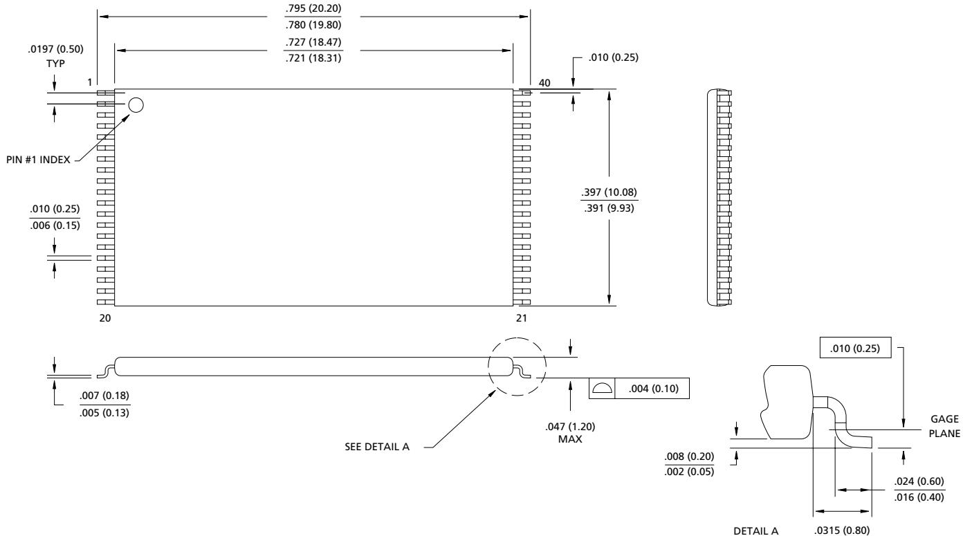
**NOTE:** 1. All dimensions in inches (millimeters) MAX or typical where noted.
