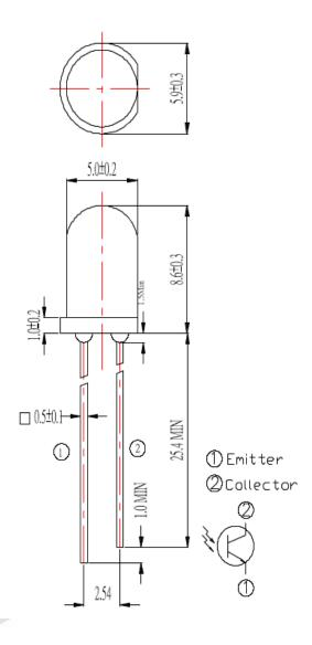
Note: Tolerances unless dimensions ±0.25mm
