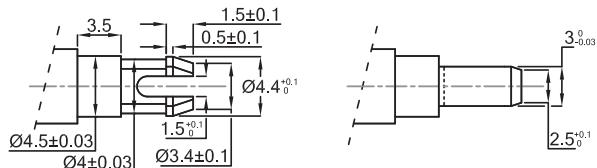
The diagram illustrates the snap-in part of a plastic actuator which can be used to rotate the Series 51 Standalone module.
