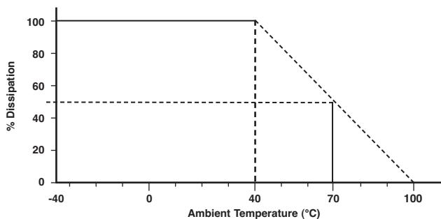
Dissipation as a function of temperature.
