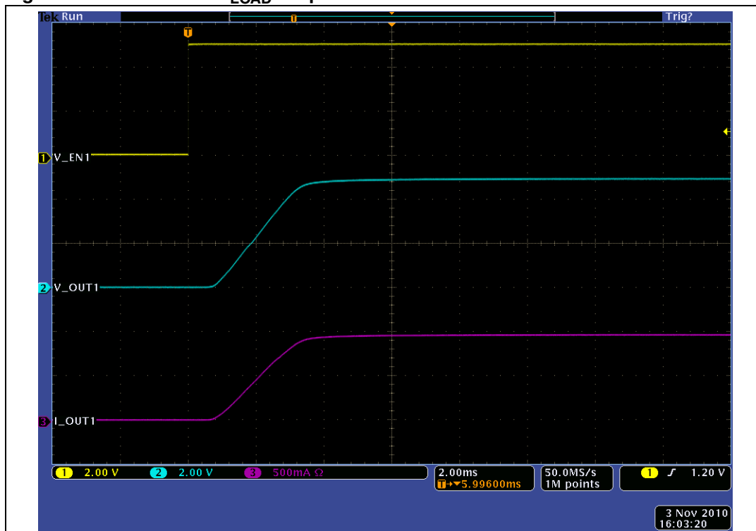
Figure 29. Turn-on for C_{LOAD} = 1 \mu F
