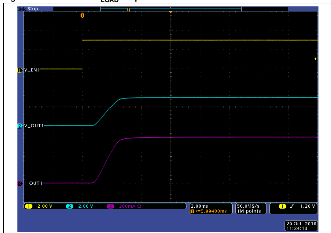
Figure 3. Turn-on for C_{\text{LOAD}} = 1\ \mu\text{F}
