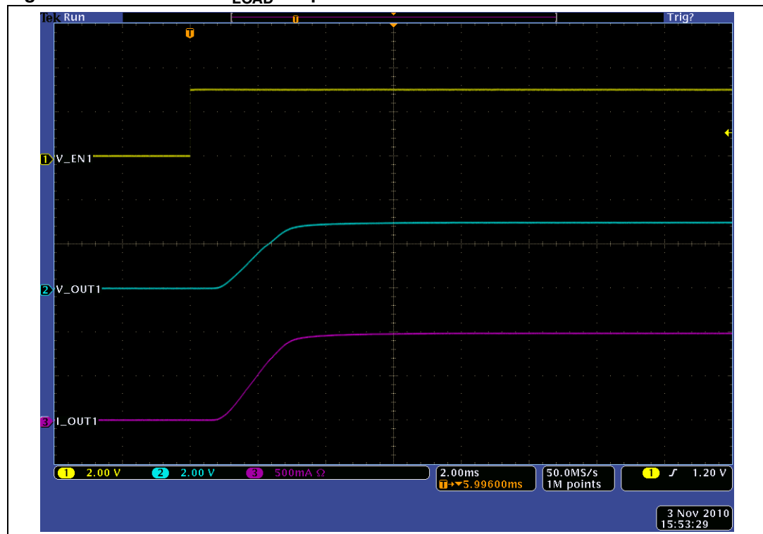
Figure 23. Turn-on for C_{\text{LOAD}} = 1\ \mu\text{F}
