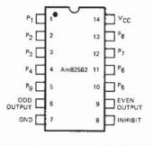
Note: Pin 1 is marked for orientation.
