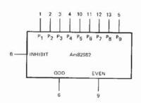
V<sub>CC</sub> = Pin 14 GND = Pin 7
