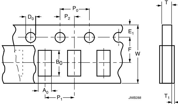
**DIMENSIONS OF PAPER TAPE** in millimeters
