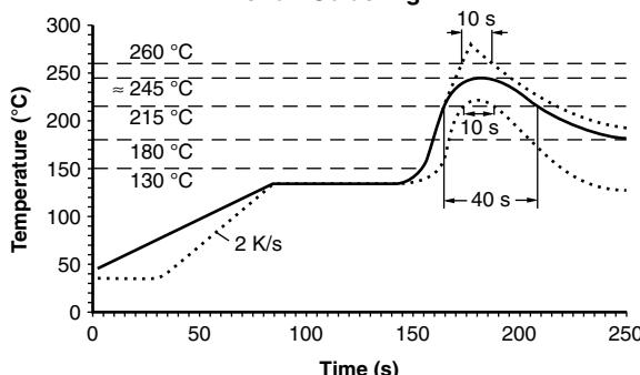
**Lead (Pb)-free Reflow Soldering Profile**
