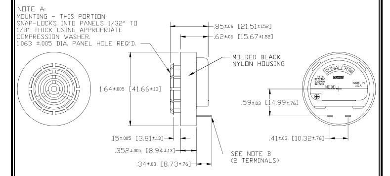
NOTE B: TERMINALS - .022 BRASS, HOT TIN FINISH WITH .065 WIRE HOLE. TERMINAL WILL ACCEPT STANDARD 1/8" QUICK CONNECT
