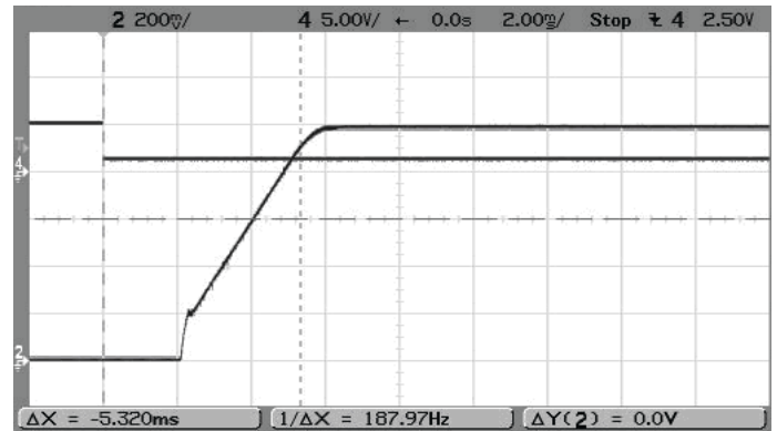
Step Load Transient Response (Vin=5V, Vout=1.0V, Load=0, Iout=3A to 1.5A) Trace 2=Vout, 100 mV/div. Trace 4=Iout, 2.5A/div.
