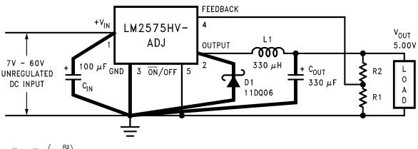
$V_{OUT} = V_{REF} \left( 1 + \frac{R2}{R1} \right)$
