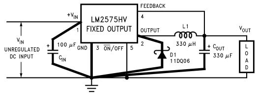
$C_{\text{IN}}$  — 100  $\mu\text{F}$ , 75V, Aluminum Electrolytic
