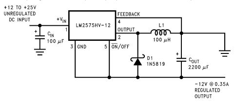
Figure 32. Inverting Buck-Boost Develops -12V
