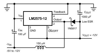
Typical Load Current 200 mA for  $V_{\rm IN} = -5.2 \rm V$  500 mA for  $V_{\rm IN} = -7 \rm V$  Pin numbers are for TO-220 package.
