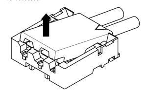
Slift up to the upper direction and positive lock is released. Removal completes.
