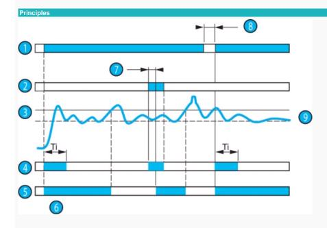
When the HSV has been configured in "memory" mode, if overspeed is detected, the output relay stays in the rest state ("alarm") irrespective of any subsequent change in the speed of the process. It will not be able to revert to ("normal") operating state until contact S2 closes (50 ms minimum). If, when S2 reopens, the speed is too high, the relay reverts to the rest latched state
