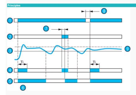
When the HSV has been configured in "memory" mode, if underspeed is detected, the output relay stays in the rest state ("alarm") irrespective of any subsequent change in the speed of the process.
