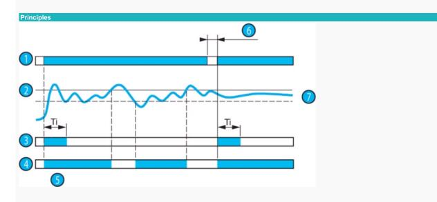
After the end of the inhibit delay on starting, "Ti", as soon as the measured speed rises above the threshold value, the output relay changes state, from operating point to rest position ("alarm" operational state, 11-14 open and 11-12 closed).
