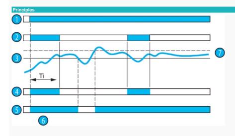
On energisation, to allow the controlled process to reach its nominal operating speed, the HSV relay is inhibited for a period that is adjustable from 0.6 to 60 seconds.
