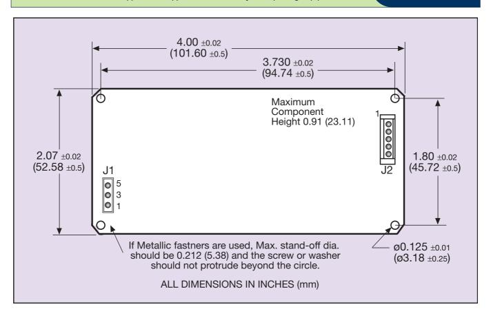
Input and output connectors Mating connectors
