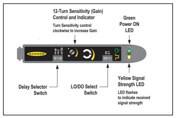
Figure 1. D10 Bipolar Discrete sensor features
