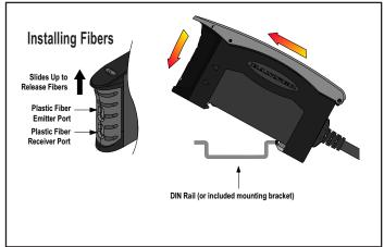
Figure 2. Installing D10 fibers and housing
