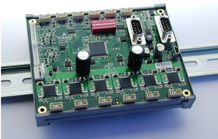
Figure 3.2 DIN rail mounting
