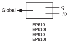
Figure 3. Classic Feedback Multiplexer Configurations
