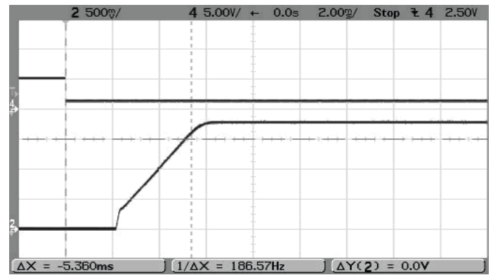
On/Off Enable Startup ( V_{IN} = 5V , V_{OUT} = 1.8V , I_{OUT} = 6A , Load=0) Trace 4=Enable, Trace2=Vout
