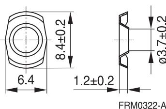
**Insulating washer 2**
