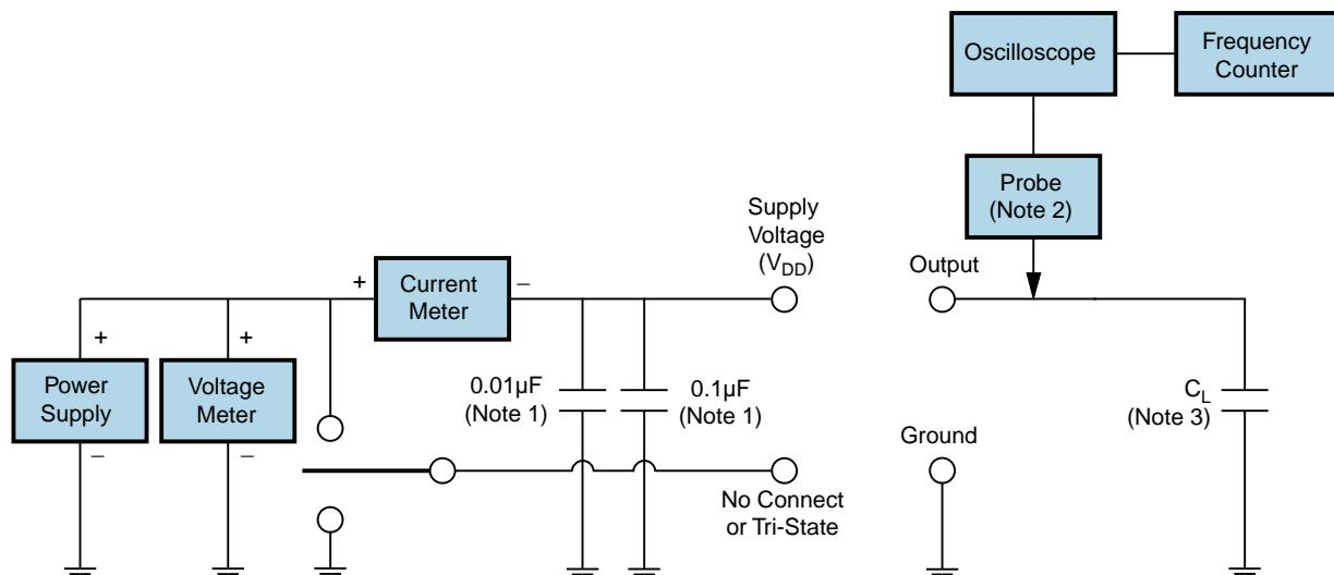
Note 1: An external  $0.1\mu\text{F}$  low frequency tantalum bypass capacitor in parallel with a  $0.01\mu\text{F}$  high frequency ceramic bypass capacitor close to the package ground and  $V_{DD}$  pin is required.
