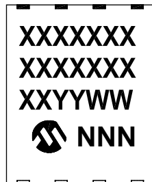
8-Lead DFN-S (6x5x0.9 mm)
