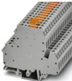
Knife disconnect terminal block, With test socket screws for insertion of test plugs, nom. voltage: 400 V, nominal current: 26 A, connection method: Screw connection, cross section: 0.2 mm<sup>2</sup> - 4 mm<sup>2</sup>, AWG: 24 - 12, length: 80 mm, width: 6 mm, color: gray, mounting: NS 35/7,5, NS 35/15, NS 32
