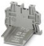
Quick mounting end clamp for NS 35/7,5 DIN rail or NS 35/15 DIN rail, with marking option, with parking option for FBS...5, FBS...6, KSS 5, KSS 6, width: 5.15 mm, color: gray
