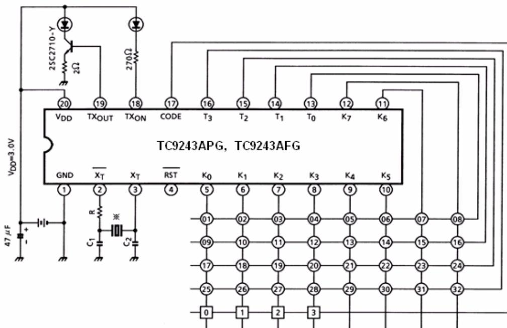
Note 4: Ceramic oscillator CSB455E (Murata Seisakusho)  $C_1 = C_2 = 100 \text{ pF}$   $R = 6.8 \text{ k}\Omega$
