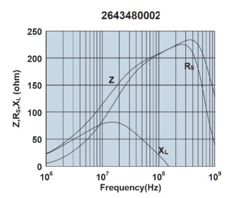
Impedance, reactance, and resistance vs. frequency.
