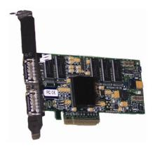
An integral member of the QLogic family of interconnect offerings, the 7104-HCA-*xxx* series Single Data Rate (SDR) HCA is a single or dual port 4X IB HCA utilizing a x8 PCle interface to enable higher server bandwidth than is possible with PCI-X. It offers an aggregate to 20 Gbps of full-duplex bandwidth.
