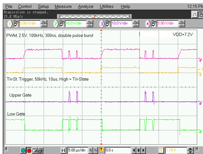
Figure 21. 2.5-V Amplitude PWM Pulse
