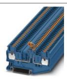
Knife disconnect terminal block, Connection type: Push-in connection, Cross section: 0.14 mm² - 4 mm², AWG: 26 - 12, Nominal current: 16 A, Nominal voltage: 400 V, Length: 70.1 mm, Width: 5.2 mm, Color: blue, Assembly: NS 35/7,5, NS 35/15
