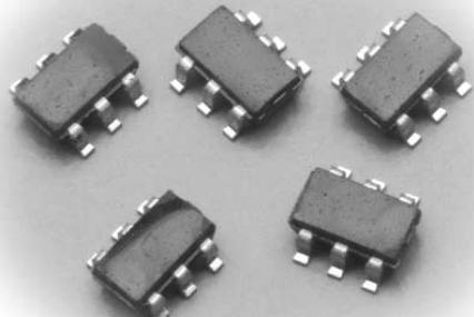
This diode network is designed to provide four channels for active termination of high-speed data signals to eliminate signal undershoot and overshoot. The network has the added benefit of acting to suppress any ESD voltage events by shunting the energy to ground assuring maximum reliability of electronic systems in the field. Trigger levels are defined by the positive and negative bias levels set by the user.
