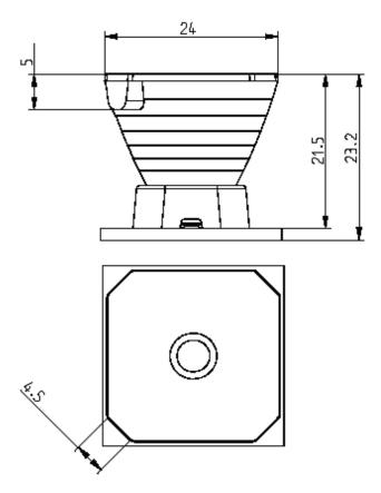
The outside mechanical dimensions of the lenses (Narrow, Medium, Wide, and Elliptical beam) are the same, except the height and top surface pattern of the lens.
