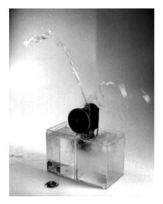
TiNi Alloy Company's TiNi-1 Engine (c 1980) uses a single coil of nitinol wire and can develop speeds of 1000 RPM on just hot and cold water.
