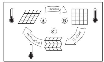
The crystal structure of a Shape Memory Alloy (SMA) such as nitinol deforms easily when below Af, its transition temperature (A). Heating to above Af causes a phase change and the alloy returns to the original shape (B) with a large force — several times greater than the force needed to deform it. When again cooled below Af, the phase change reverses (C) and it can again be easily deformed. From the "Muscle Wires Project Book" (Mondo-tronics)
