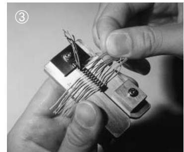
3. Arrange the wires one at a time through holding plates (A) and (B).
