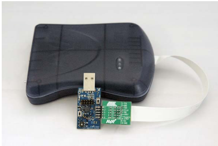
Figure 20. Connecting AVR JTAGICE mkII to the AT88Microbase
