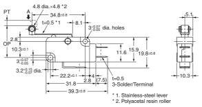
D2MV-1L2-1C3 Model Operating D2MV-01L2-1C3 characteristics Operating Force OF Max 0.29N {30 gf} Releasing Force  $\mathsf{RF}$ Min. 0.02N {2 gf} (reference value) PT Max Pretravel 3.3 mm Overtravel OΤ Min. 2.1 mm Movement Differential MD Max 0.7 mm Operating Position OP 20.7±1.2 mm
