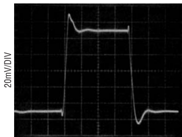
Small-Signal Transient Response V_S = \pm 2.5V
