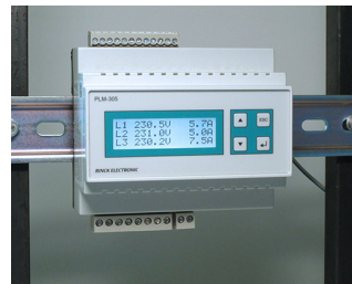
Power measuring device for energy analysis
