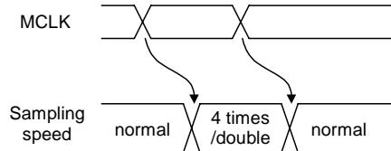
When sampling speed mode is changed between double and 4 times speed mode, sampling mode should be changed to normal speed mode after changing MCLK frequency, and then it should be changed to double/4 times speed mode (figure below). Some click noise occurs at those changing timing.
