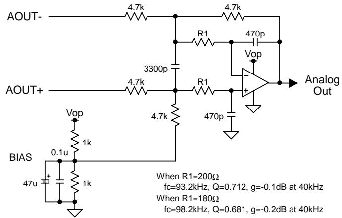
Figure 10. External 2<sup>nd</sup> order LPF Circuit Example (using op-amp with single power supply)
