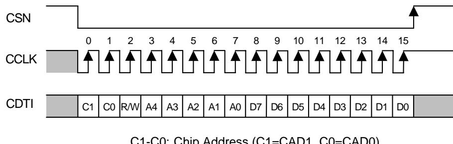
Figure 7. Control I/F Timing
