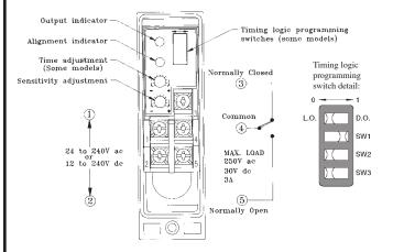
The output timing logic function (on sensor models with T9 model number suffix) is selected at the timing logic programming switches, according to the table (right). The output timing logic delays are set at
