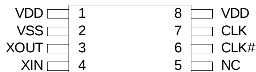
Figure 1. Pin Diagram - 8-Pin TSSOP
