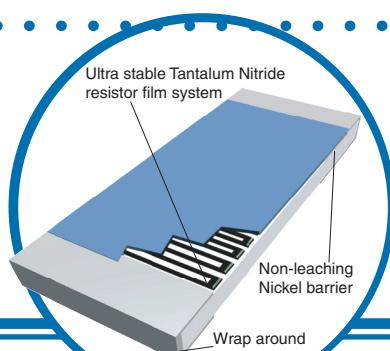
The IRC TaNFilm® PFC chip resistor series provides the high precision and ultra stable performance of our Tantalum Nitride resistive film system in 0402, 0603, 0805, 1206, 1505, 2010 and 2512 sizes. The unique characteristics of the passivated Tantalum Nitride film insure long term life stability and stability in most environments.
