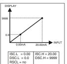
reverse scaling parameter as YES. In this case referring the above eg. for 0.00 mA input the display will show 9999 and 20.00 mA input the display will show 0.0.
