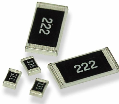
**Note:** SMD (Surface mount devices) resistors and inductors should be kept in their original packaging to protect them from ESD (Electrostatic Discharge). The full reels can be broken into smaller quantities, without exposing them to ESD, as long as the components are still in the plastic or paper tape. These resistors and inductors should not be removed from the plastic or paper tape unless they are in an ESD protected environment.
