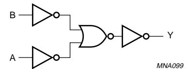
Fig.4 Logic diagram (one driver).
