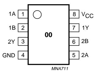
Fig.1 Pin configuration.
