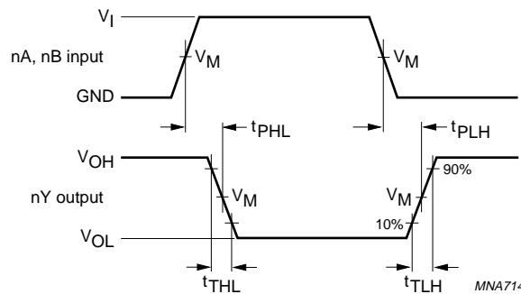
For 74HC2G00:  $V_M = 50\%$ ;  $V_I = \text{GND to } V_{CC}$ .For 74HCT2G00:  $V_M = 1.3 \text{ V}$ ;  $V_I = \text{GND to } 3.0 \text{ V}$ .
