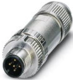
Sensor/actuator connector, male, straight, 5-pos., M12 SPEEDCON, shielded, A-coded, spring-cage connection, metal knurl, cable cross section max. 8 mm
